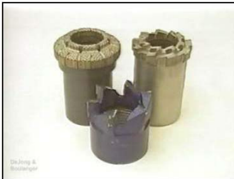
Coring Bits. From left to right: Diamond, Carbide, & Sawtooth.
